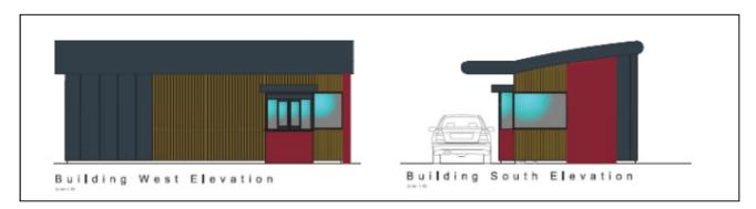
The kiosk itself (shown above) would have a rectangular footprint of 36.8m<sup>2</sup>. It would have a monopitched roof metal roof with an eaves height of 3.2 metres rising to 4 metres at its apex. The walls would be finished in black metal and composite cladding. The building would accommodate a kitchen/preparation area, service window, storage area and toilet. A bin store would stand adjacent to the building's southern elevation.
